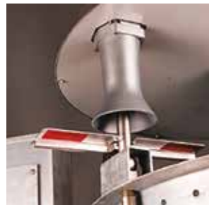
Positive fail-safe latching
